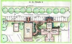
Doug's key point was that the solution at the library was a grade based ADA compliant walk which did not require ramps and railings, nor the use of Trex or aluminum. The solution was complimentary to the historic building.
